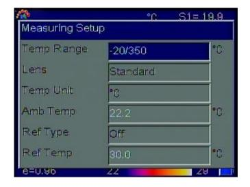
Press **Menu** key to activate the main menu. Select Setup->MeasureSet and press **Confirm** key to pop up the Measuring Setup dialog box. User can view or set temperature range, lens type, temperature unit, ambient temperature, reference type and reference temperature. Press **Up** and **Down** keys to choose different items, **Left** and **Right** keys to modify the item contents.
