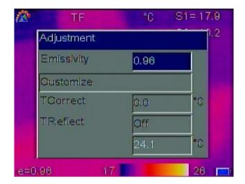
Press **Menu** key to activate the main menu. Select **Setup->Adjustment** and press **Confirm** key to pop up the Adjustment dialog box. User may set emissivity, temperature correct and ambient temperature. Press **Up** and **Down** keys to choose different items, **Left** and **Right** keys to modify the item contents.
