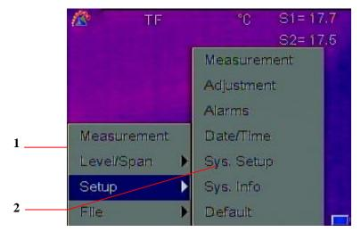
[1] Main menu: Displays four options: Measurement, auto/manually, Setup,
