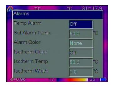
Press **Menu** key to activate the main menu. Select **Setup**->**Analysis setup** and press **Confirm** key to pop up the Analysis dialog box. User can set temperature alarm, alarm temperature, alarm color, isotherm color, isotherm temperature and isotherm width. Press **Up** and **Down** keys to choose menu items, **Left** and **Right** keys to modify the item contents.
